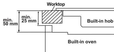
If the oven is installed under a hob, the distance between the worktop and the top panel of the oven must be minimum 50 mm and the distance between the worktop and the top of control panel must be minimum 25 mm.
