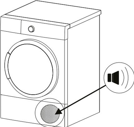
A line drawing of a front-loading washing machine. A circular area at the bottom front is circled, with an arrow pointing to a speaker icon. The speaker icon is a black trapezoid with two curved lines to its right, indicating sound. | <p><b>Som do Compressor</b></p> <p>É normal ouvir um som metálico do compressor de vez em quando, enquanto a máquina está em funcionamento.</p>                                                              |
